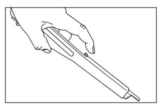
3. Extend the handle on the wheel wrench by pressing the button with your index finger and pulling on the end of the wrench. You must do this before using the wheel wrench.
